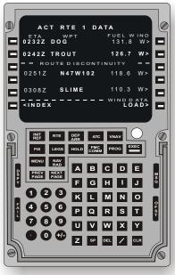
Once the route of flight is activated, Request the WINDS. push LOAD> (6R)
