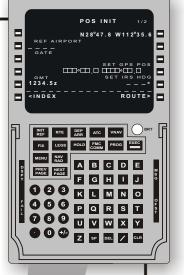
The FMCS validates the integrity of the GPS signal source. A successful completion of the validation process results in the display of position data at 4R.
