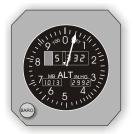
Ensure that the STANDBY ALTIMETER has the correct barometric setting. Specifically notice whether hectropascals or inches of mercury are applicable. During the approach, monitor the CDU LEGS PAGE for specific distance, heading, and fix information.
