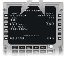
Using the **EFIS**, the pilot can select the **VOR** or **ADF** displays on the **ND** (Navigtion Display).
