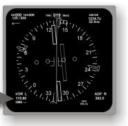
Throughout the approach, even while using the LNAV and AUTOPILOT; it is good technique to be constantly "Marrying the bugs" (setting the HDG SEL bug on the ND to the heading desired) so that should a transition to HDG SEL become necessary, the MCP will be set up and the airplane will not make a turn off course.
