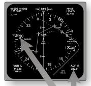
BOTH PILOTS must be is the MAP mode, either CTR or EXPANDED. I have depicted using the CTR mode on the
