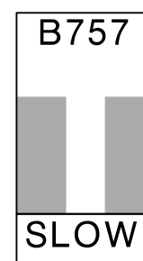
The system goes into "downgrade" mode due to bad weather conditions, pilot will be promoted to slow down. Docking process will continue when the aircraft is detected but pilot should exercise caution
